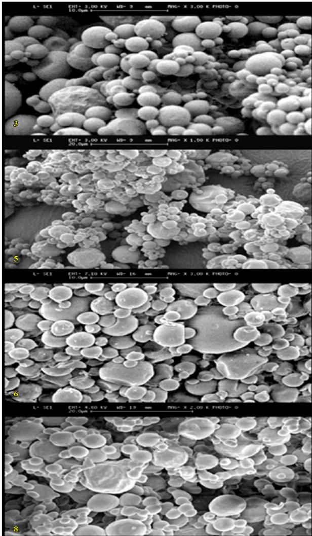
Figure 3. The scanning electron micrographs for barberry extract powder, while different level of MD:AG were used as the drying aid (samples 3,5,6,and 8)
